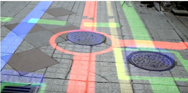
Evaluating the potential of the Microsoft HoloLens for displaying vertical projection of subsurface utility pipes on the road surface.
