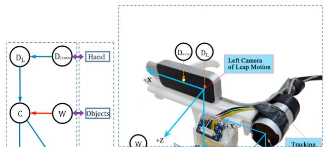
Figure 5. The structure of the proposed system: The relationship between the coordinate systems (left). The correspondence between the symbols and the components (right).
