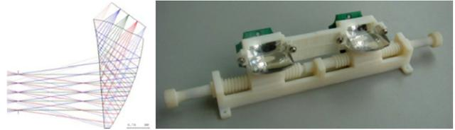
Figure 3. The eyepiece design layout and the HMD prototype assembly.
